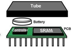
These transitions to and from the external power source does not affect the SRAM, making it a true nonvolatile memory. This unique construction combines the strategic advantages of SRAM –addressing structure, high–speed access, and timing requirements– with the non-volatility advantages of EEPROM technologies.
